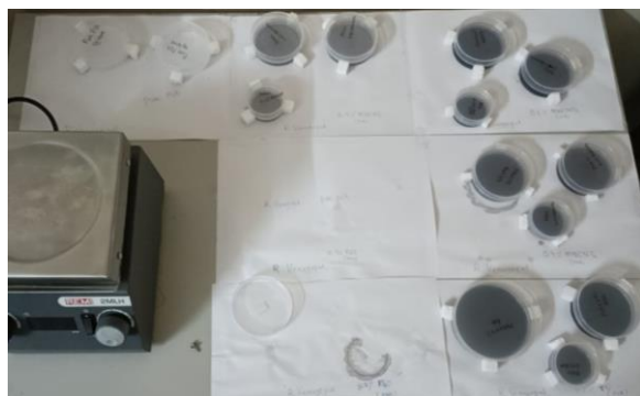
Figure 2. Stirring machine for the preparation of PVA-RGO nanocomposite films.& Images of the Prepared PVA-RGO Composite Films.
