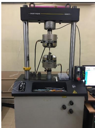
Figure 1. Compressive load application on tooth sample using universal testing machine.
