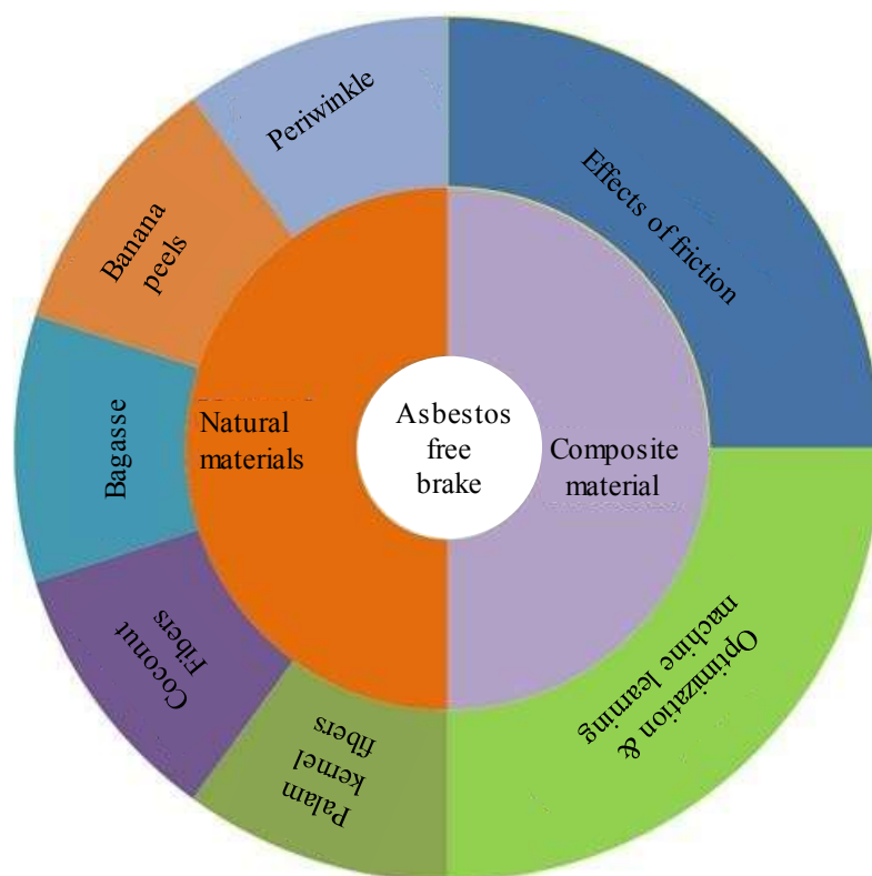
Figure 3. Categorization of Natural Materials and Composite Improvements in Asbestos-Free Brake Pads
