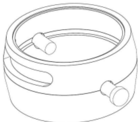
Figure 2. Isometric view of counter flask placed on base flask with rods: side view.
