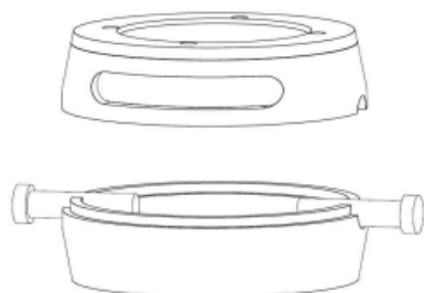
Figure 1. Isometric view of the dental flask.
