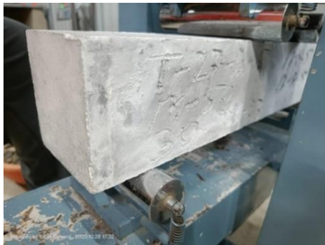
Figure 3. Test setup for flexural testing of beams.
