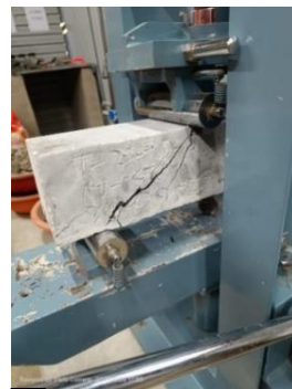
Figure 3. Test setup for flexural testing of beams.
