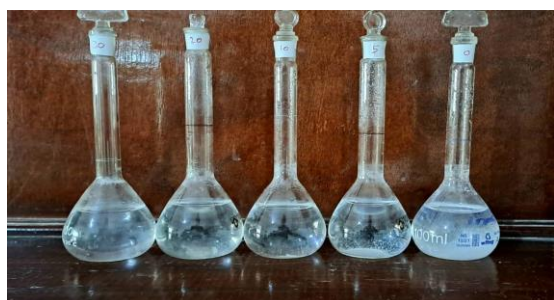
Figure 4. Scale test observation for \text{CaCO}_3 at 70^\circ\text{C} .
