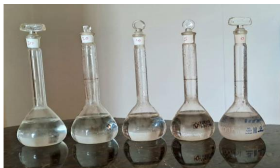
Figure 5. Scale test observation for \text{CaSO}_4 at 70^\circ\text{C} .
