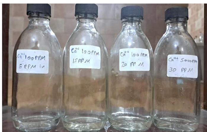
Figure 6. Compactivity test in 100 ppm \text{Ca}^{2+} and 3% NaCl in 2 mL.
