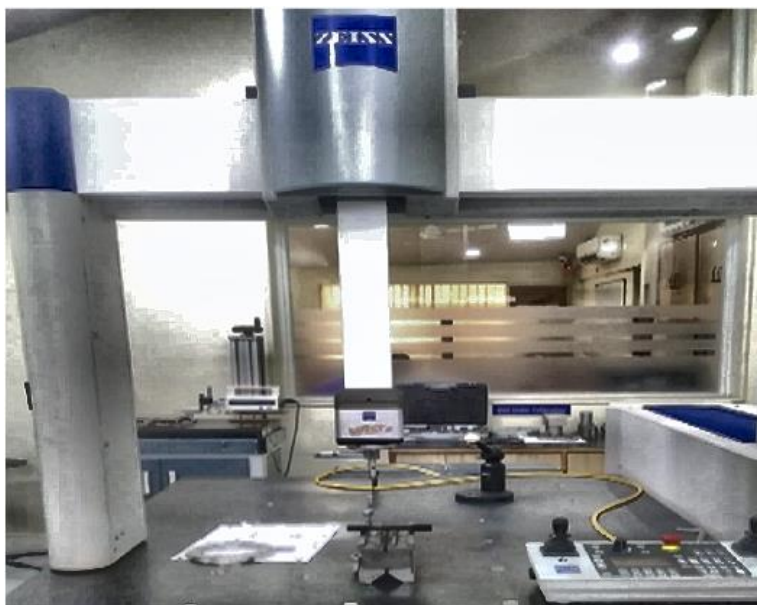
Figure 7. (b) CMM ZEISS CALYPSO used for Measurement the Specimen
