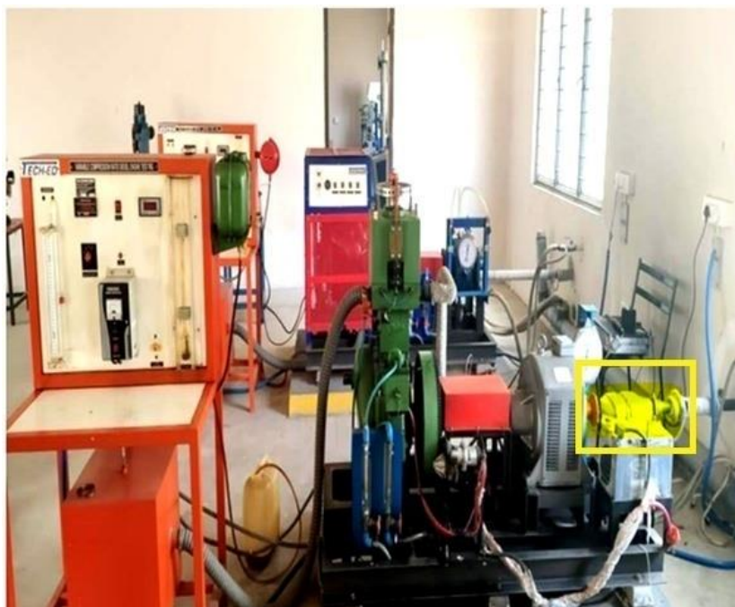
Figure 6. Four Stroke Single Cylinder Variable Compression Ratio Diesel Engine with Palladium Catalytic Converter
