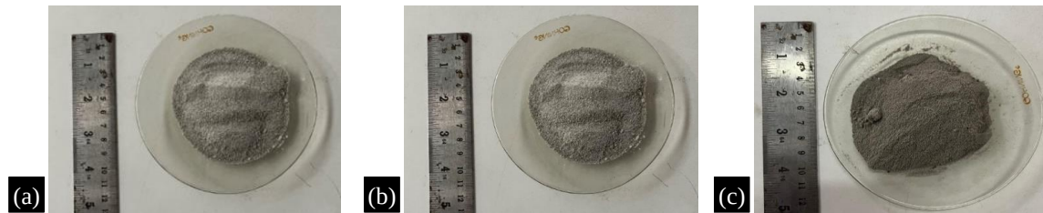
Figure 3. Different Grades of Steel Slag (a) Crude steel slag (S1) (b) 3'n Pulverized steel (c) 5'n Pulverized steel slag(S3) slag (S2)
