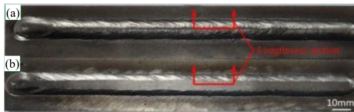
Figure 15. (a), (b) Effect of the roller on the weld bead in rolling-assisted WAAM.
