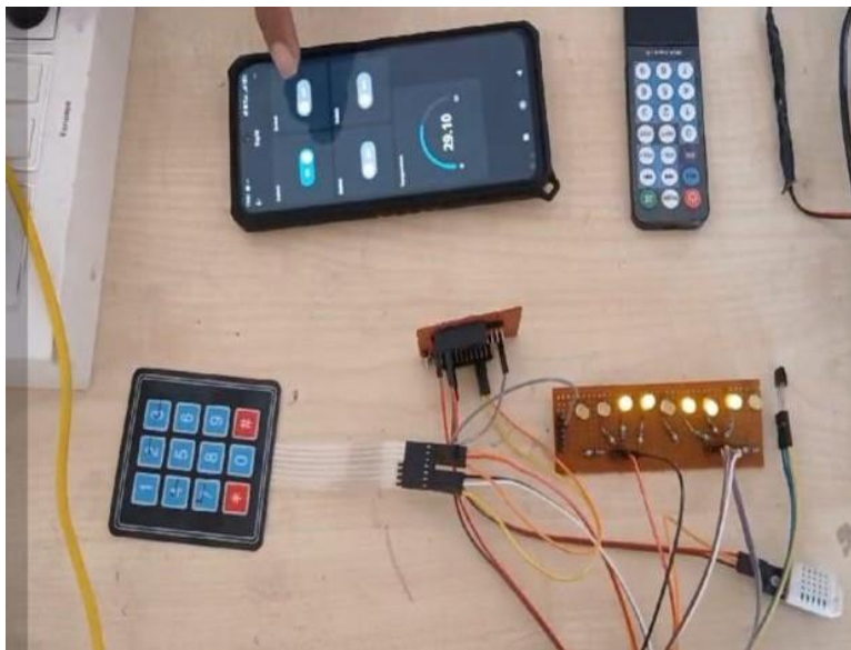
Figure 10. System operate using Arduino IoT Cloud app dashboard.
