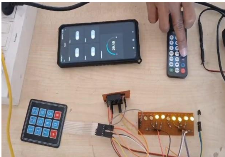
Figure 11. System operate using IR remote.
