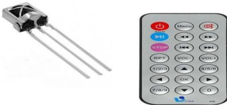
Figure 4. IR Remote and TSOP receiver.
