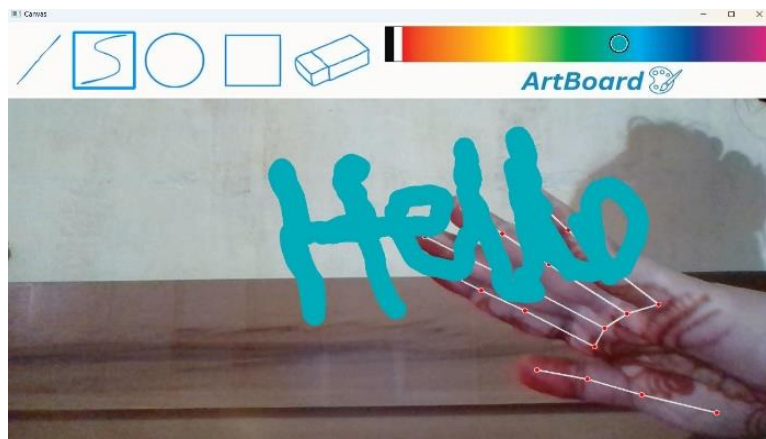
Figure 5. Freehand drawing in AirDraw captures natural finger movements to create fluid sketches on a virtual canvas.
