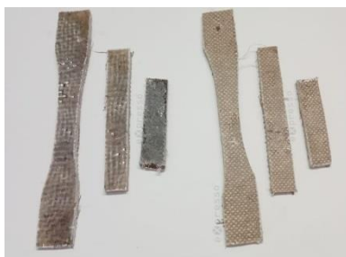
Figure 3. Hybrid and synthetic composite specimens for mechanical testing.
