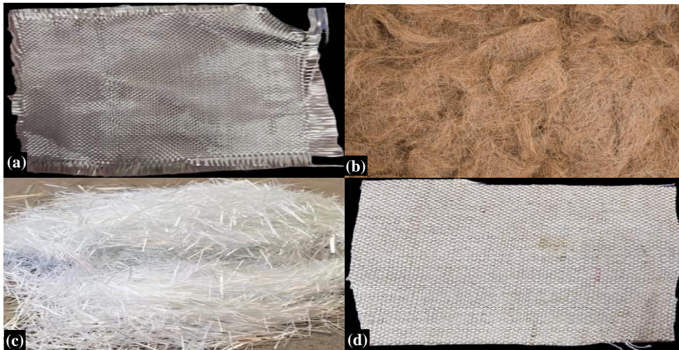
Figure 1. Materials Used for Manufacturing Composite (A – Basalt fibre B – Coconut coir C- Glass fibre D – Kenaf fibre sheet).
