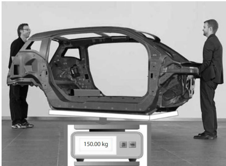
Figure 2. Demonstrable lightweight BMW i3 life module fabricated from carbon fiber composite. The total weight of each capsule was 150 kg.
