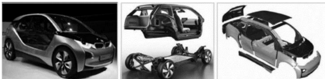
Figure 1. BMW is the first mass manufactured lightweight car with a predominant part of its structure and body manufactured from carbon fiber-reinforced composites.
