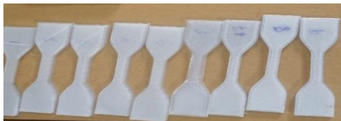
Figure4. 3D printed PETG Material Tensile specimens.
