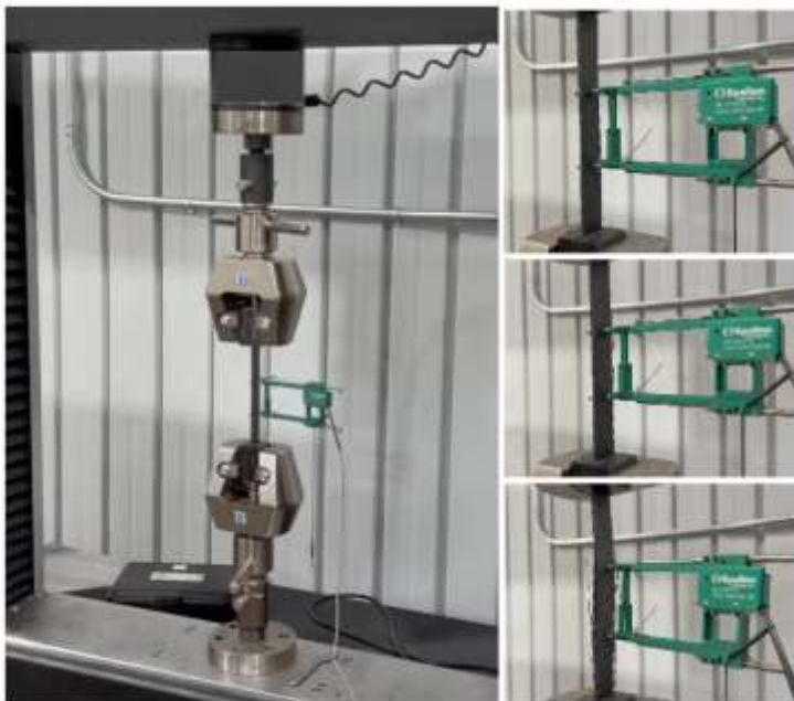
Figure 7. Fatigue strength specimen as per ASTM D3479.
