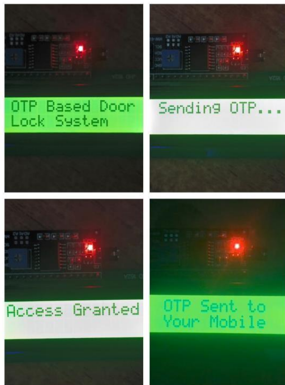
Figure 8. OTP Authentication and access verification process.
