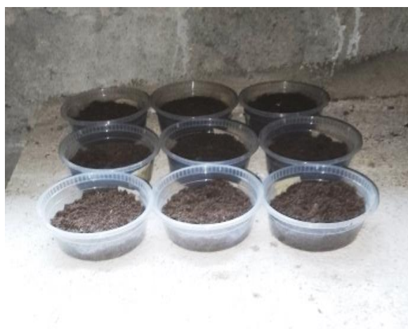
Figure 3. Experimental Set-up of bioremediation of condemn oil in loamy soil using Azadirachta Indica.
