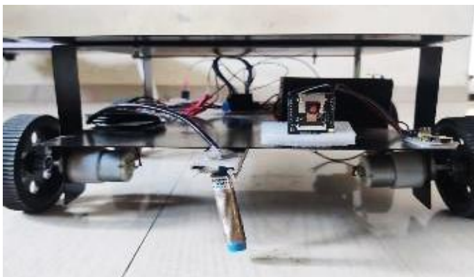
Figure 2. Rover for landmine detection.
