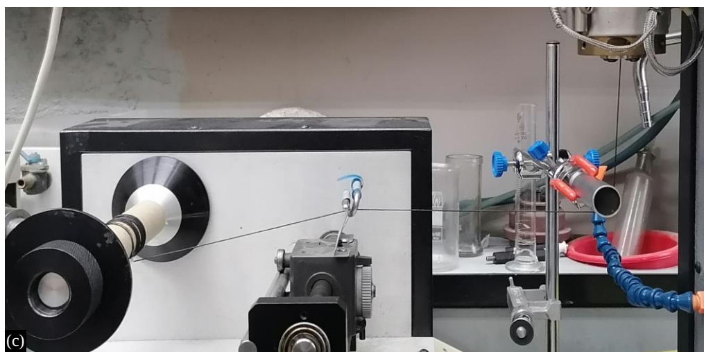
Figure 2. Images of the UHMWPE fibers (a) - before and (b) - after orientation drawing; (c) - spinning process of UHMWPE fiber containing 25 wt.% CB.
