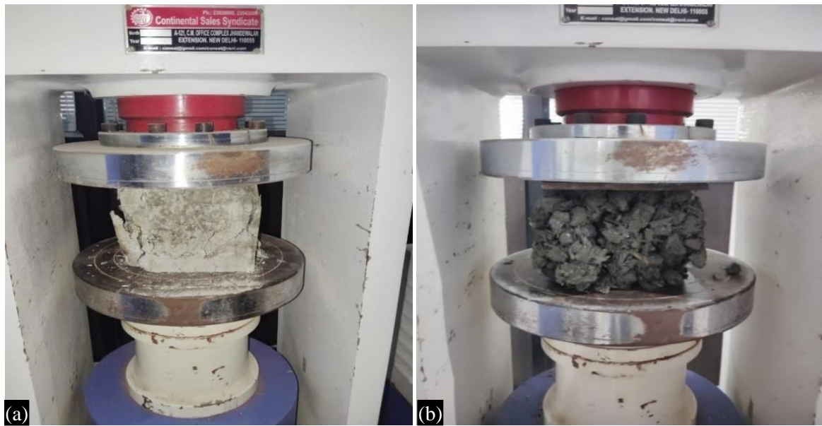
Figure 6. Specimen under failure in CTM.
