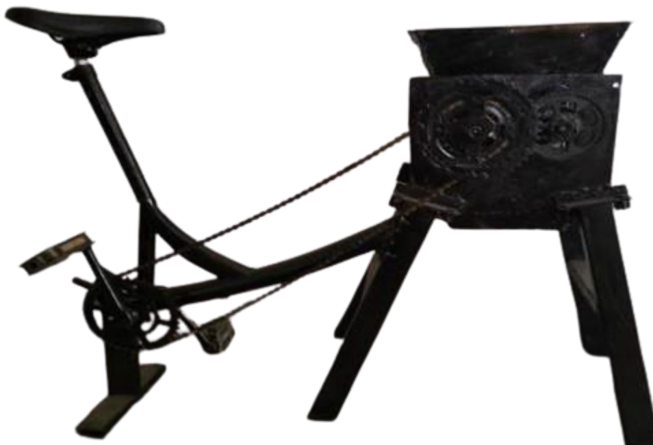
Figure 8. Pedal operated apple peeler machine.
