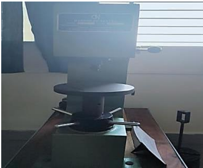
Figure 6. Brinell hardness tester machine.
