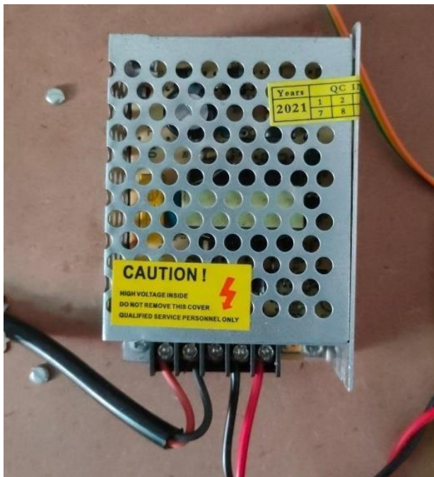
Figure 2. Switched mode power supply (SMPS).
