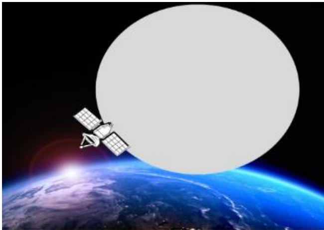
Figure 9. Inflated ball method for drag augmentation of the debris [4].
