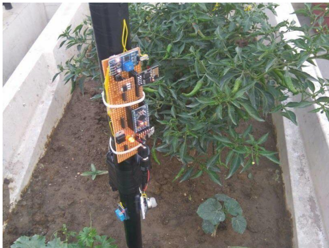
Figure 3. Actual implementation of soil fungus detection system.
