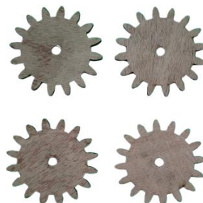
Figure 2. Four 90 mm diameter planet gear.
