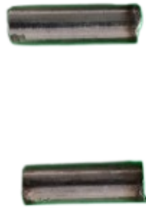
Figure 4. 200 mm steel rods (8 mm diameter).
