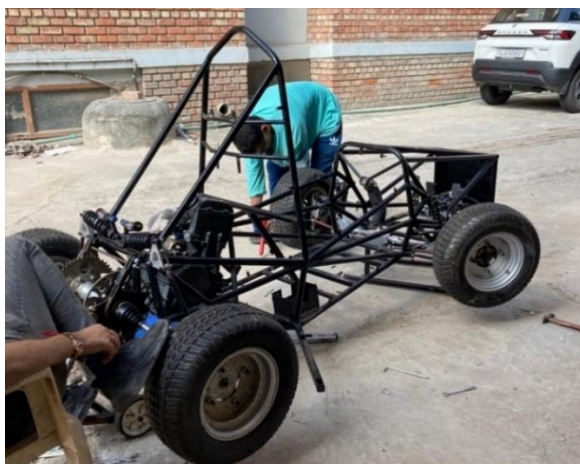
Figure 17. Manufactured chassis and drivetrain.
