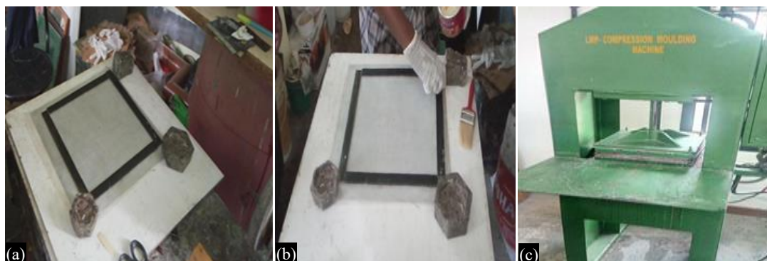
Figure 1. (a) Hand lay method of deposition; (b) Mold set up; (c) Press with die assembly.
