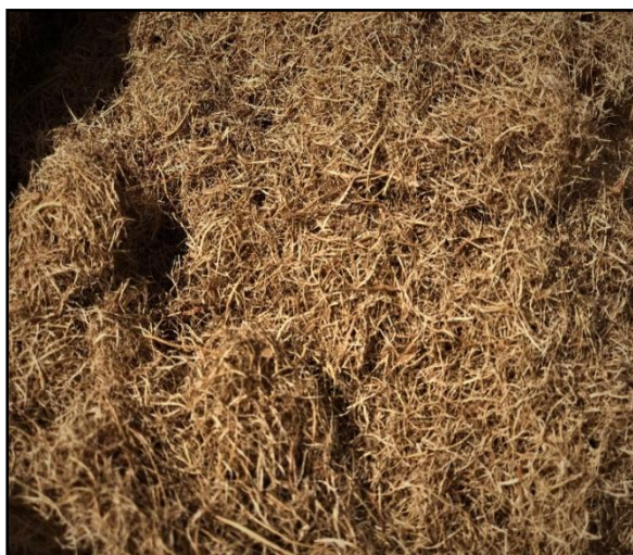
Figure 1. The short random oil palm empty fruit bunch (OPEFB) fibres utilized in this experimental research.
