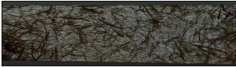
Figure 7. Specimen with a resin rich morphology.
