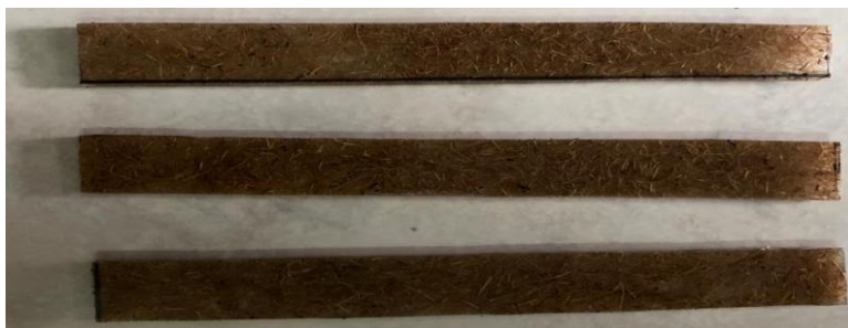
Figure 2. The oil palm empty fruit bunch (OPEFB)/epoxy specimens for tensile and hardness tests.
