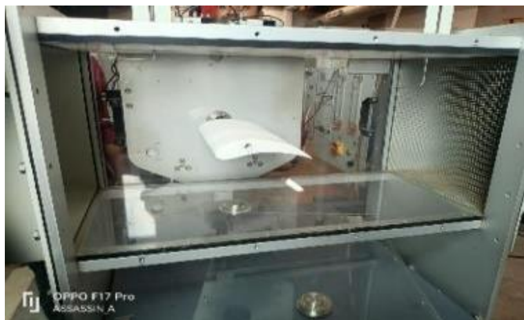
Figure 2. Testing of 3D printed airfoil in wind tunnel.
