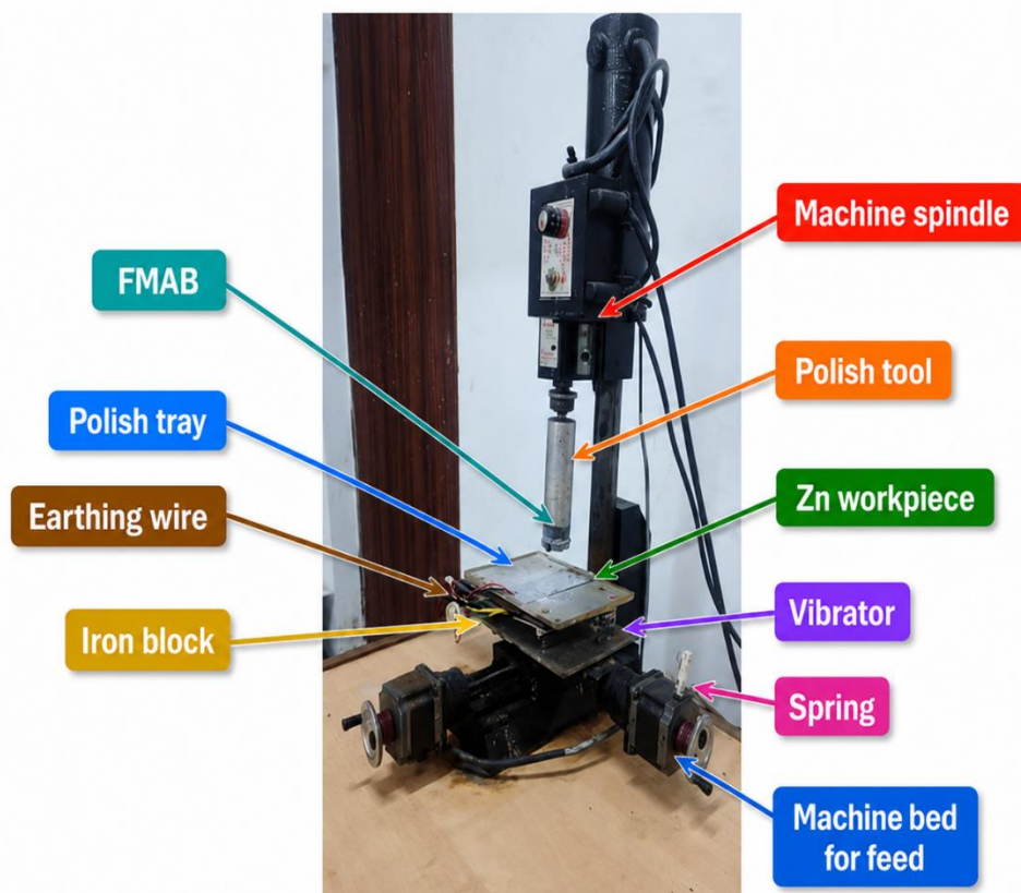
Figure 1. Detailed schematic of the UV-SPMAF experimental setup. Key components: CNC machine spindle (BFW MCV-300), NdFeB permanent magnet ( \varnothing 25 mm, N52, 0.45 T), flexible magnetic abrasive brush (FMAB: 30% \text{Al}_2\text{O}_3 + 70% Fe), zinc workpiece ( 50 \times 50 \times 5 mm), piezoelectric ultrasonic transducer (Branson 2000X, 20/40 kHz, 5–15 \mu\text{m} , Z-axis), vibrating platform with springs, iron block, polishing tray, infrared thermometer (Fluke 572-2, \varepsilon = 0.23 ), chemical polishing agent ( \text{HNO}_3 + \text{H}_2\text{O}_2 ).
