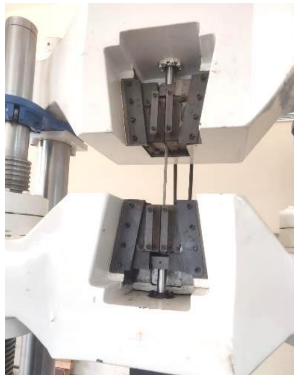
Figure 4. Tensile testing using UTM machine
