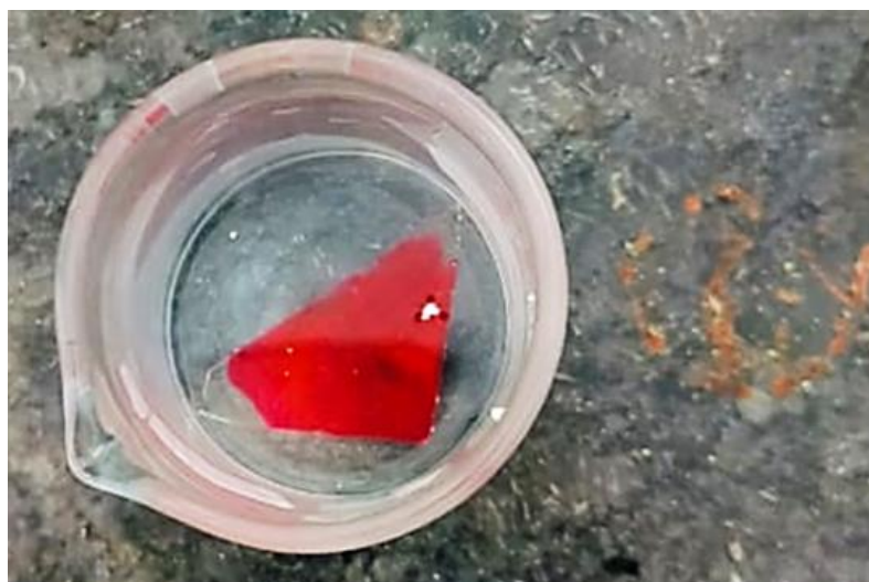
Figure 9. Water resistance test for nail lacquer.
