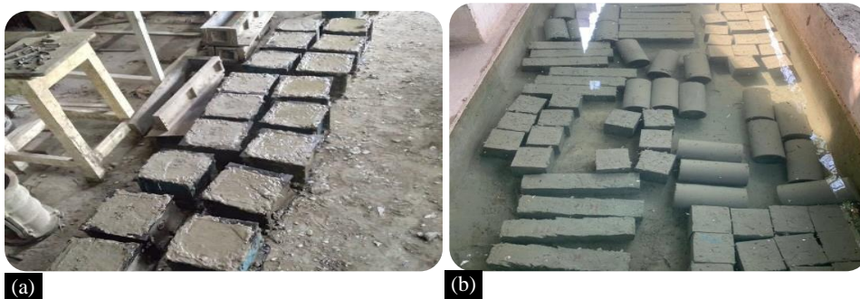
Figure 3. Photographs of a) casting of moulds and b) curing of moulds.
