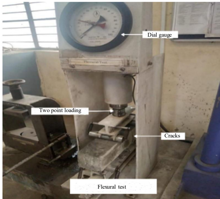
Figure 6. Concrete beam subjected to flexural strength test.
