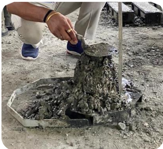
Figure 4. Illustration of slump cone test.
