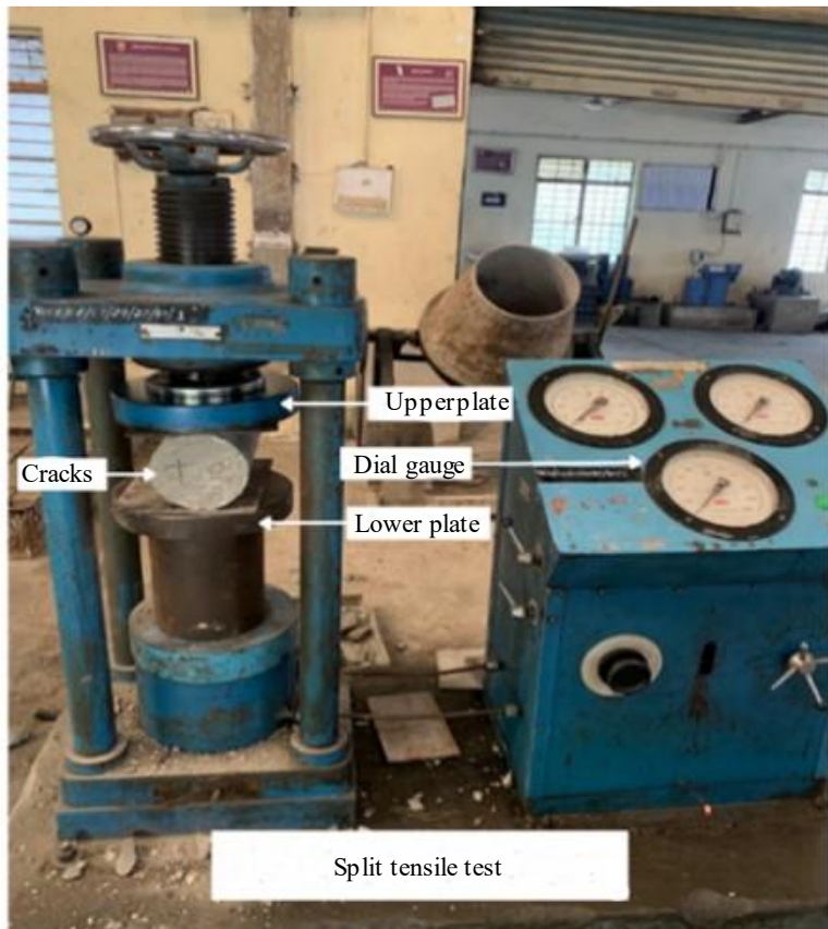
Figure 7. STS on cylindrical specimens.
