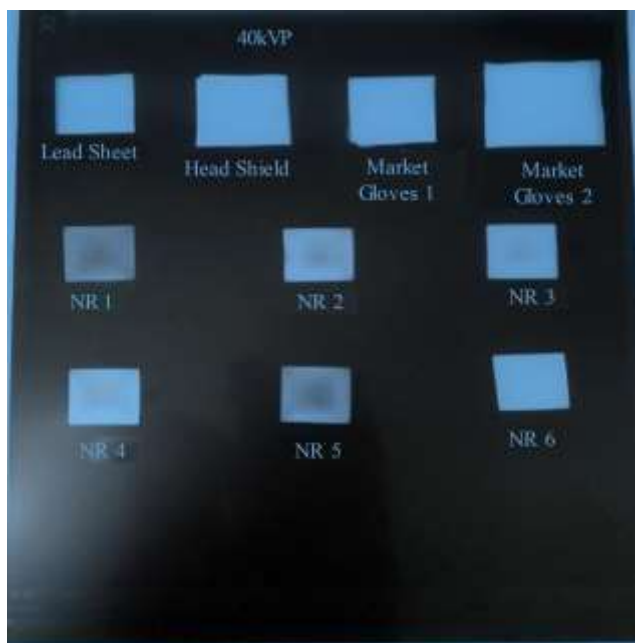
Figure 5. X-ray Radiograph of E-Waste-Rubber Composite
