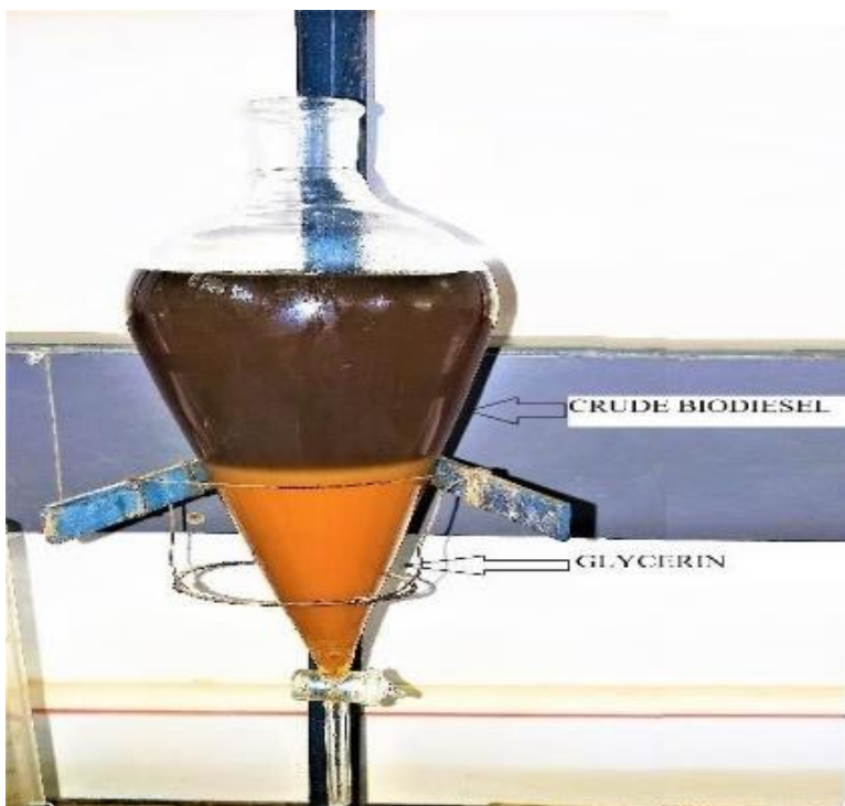
Figure 5. Crude biodiesel after transesterification
