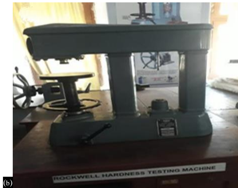
Figure 1. (A) Experimental Setup (B) Rockwell Hardness Testing Machine
