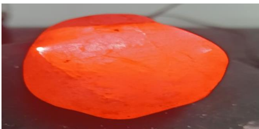
Figure 11. Natural Luminescent stone under Red Laser light of wavelength 650 nm.
