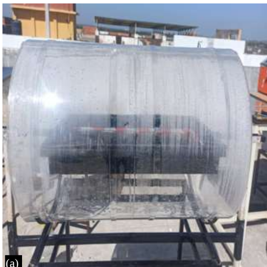
Figure 4. (a) and (b) Photograph of experimental setup FRP composite material CTSS and MTSS solar still [10].
