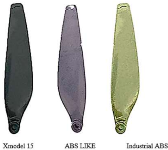
Fig. 3 – Different 3-D printed materials used in UAVs
