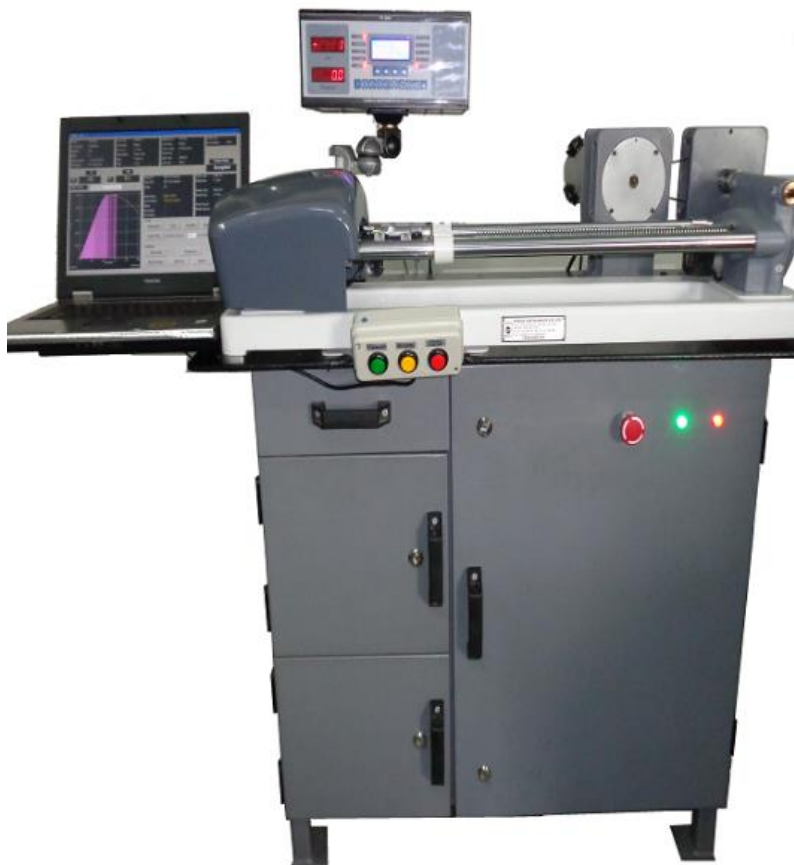
Figure 5. Tenso meter test machine (PC2000).
