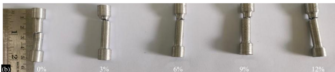
Figure 11. Tensile strength specimen (a) with copper chills and without water circulation after experiment, (b) with copper chills and with water circulation after experiment.
