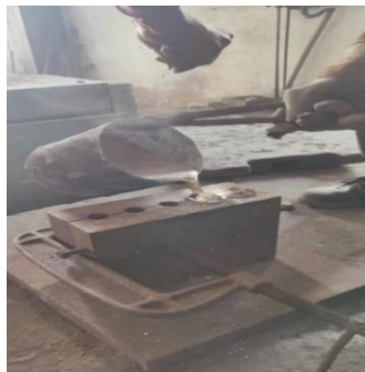
Figure 3. Pouring of molten metal.
