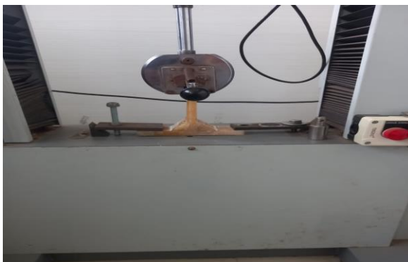
Figure 6. Composite T joint mounted on UTM for Tensile test.
