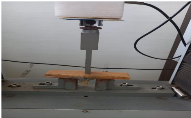
Figure 10. Three-point bending test on composite T joint.
