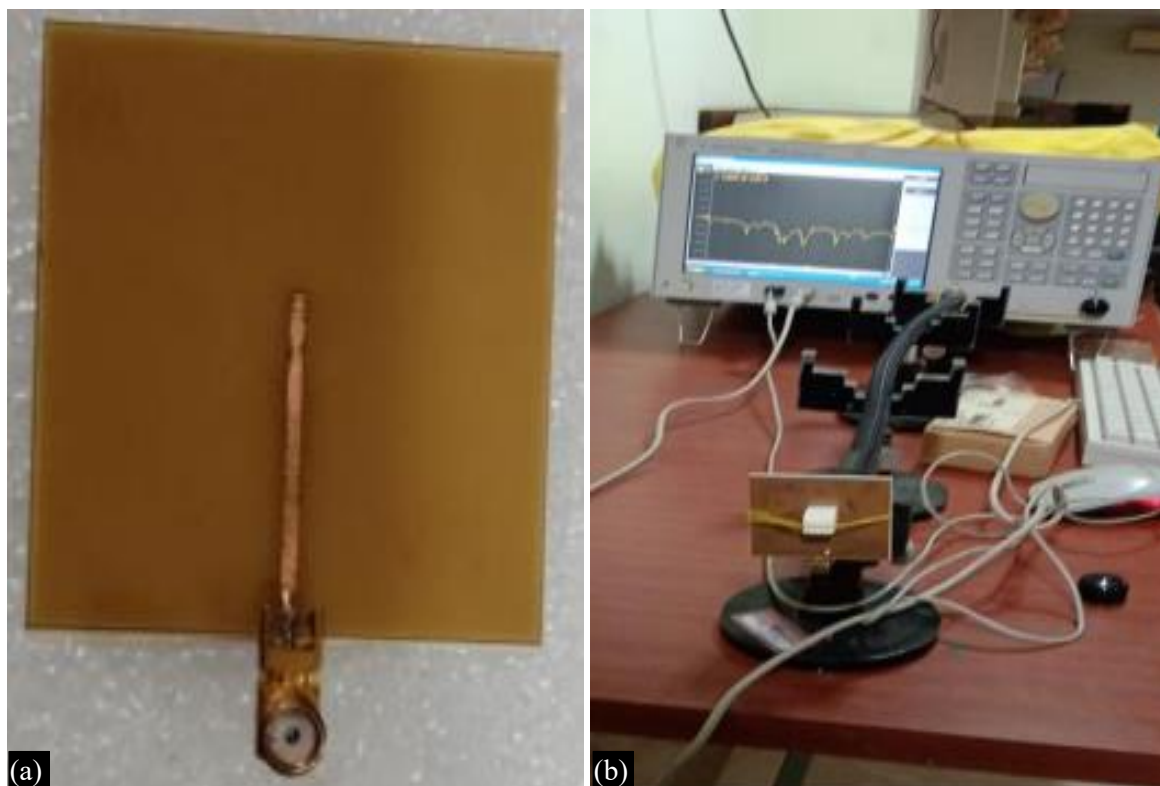
Figure 3. (a) Koch slot array antenna; (b). Antenna with power supply.
