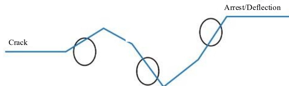
Figure 7. Crack Arrest Mechanism by Reinforced Particles in Polymer Composite Interlayer
