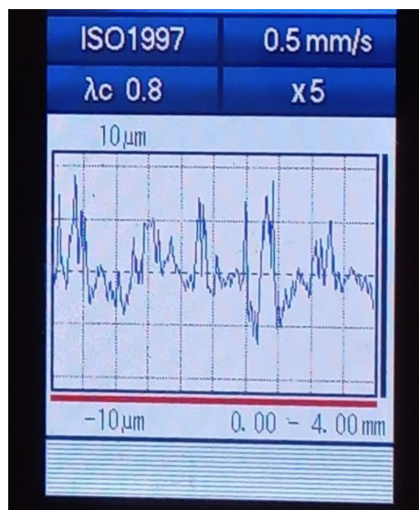
Figure 8. Results of surface roughness.
