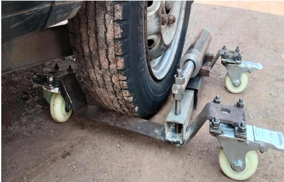
Figure 6. Car moving kit testing on Maruti Suzuki 800.
