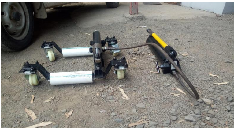
Figure 5. Assembly of car moving kit with cylinder.
