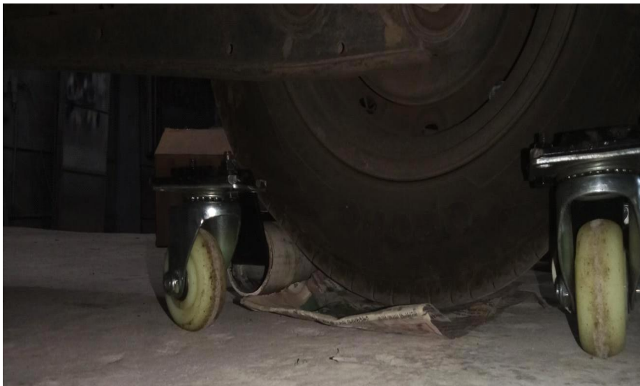
Figure 7. Testing of easy car moving kit on Maruti Alto 800.
