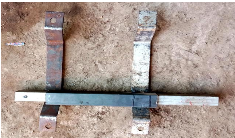
Figure 4. Assembly of car moving kit frame.
