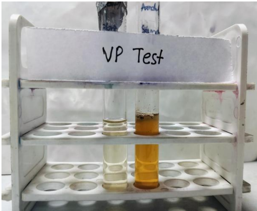
Figure 6. Strain is showing red color which indicates they form acetoin.
