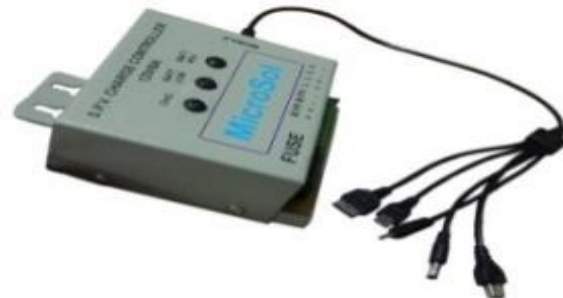
Figure 3. Solar charge controller [9].
