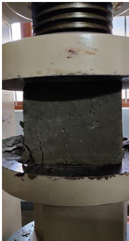
Figure 6. Testing of SCCC specimen (source:pic taken at PVPSIT).
