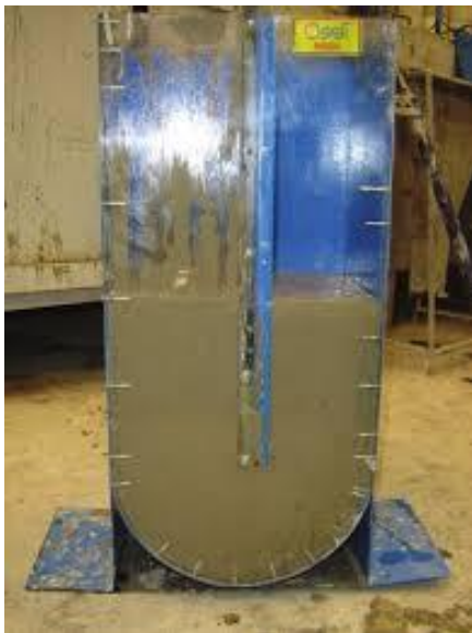
Figure 5. U-Box Test for Self-Compacting Composite Concrete (Source: pic taken at PVPSIT).
